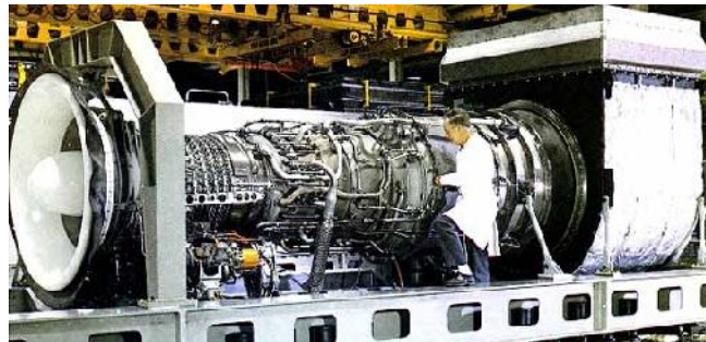
Photo 4: Gas turbine as compressor drive
