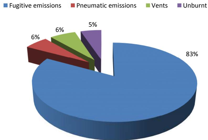
*Figure 2: Methane emission sources from LNG terminals with flare*
