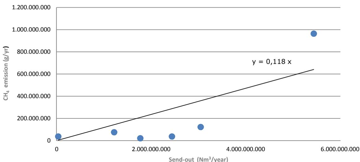
*Figure 1: Total CH<sub>4</sub> emissions (in g CH<sub>4</sub>) per LNG terminal of the 2015 representative dataset relative to each 2015 send-out*
