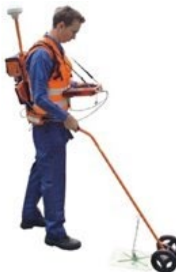
Figure 12 – Illustration of walking detection via carpet probe
