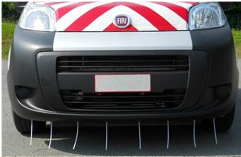
Figure 4 - Example of leak detection with car driving along buried lines. Source: MARCOGAZ' members
