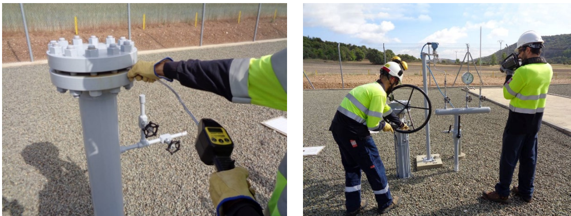
Figure 2 - Example of exercise of detection of leak at above ground asset. Source: MARCOGAZ' members
