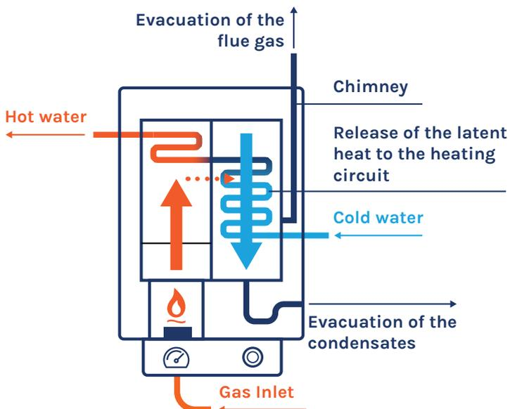
Schematic illustration of a gas condensing boiler
