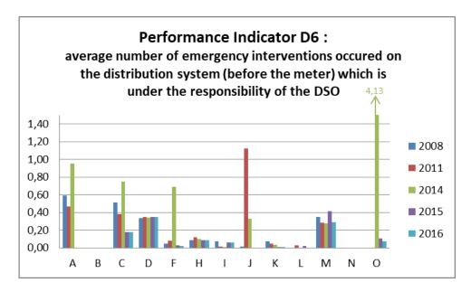
The graph shows a large disparity between the Countries. The total number of emergency interventions is much higher than the number of intervention for leaks (3 times higher). Explosion, fire, lack of gas, pressure drop or excess of pressure are the main reasons for interventions.
