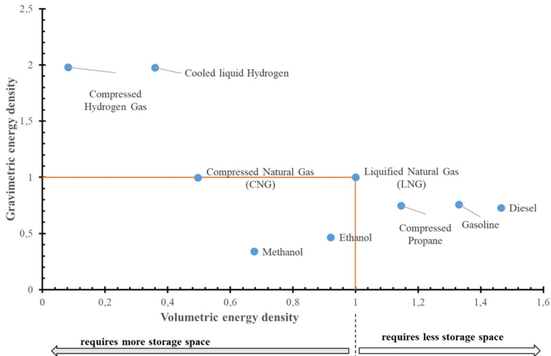
Figure 1 - Energy density comparison of several transportation fuels (gasoline = 1).
