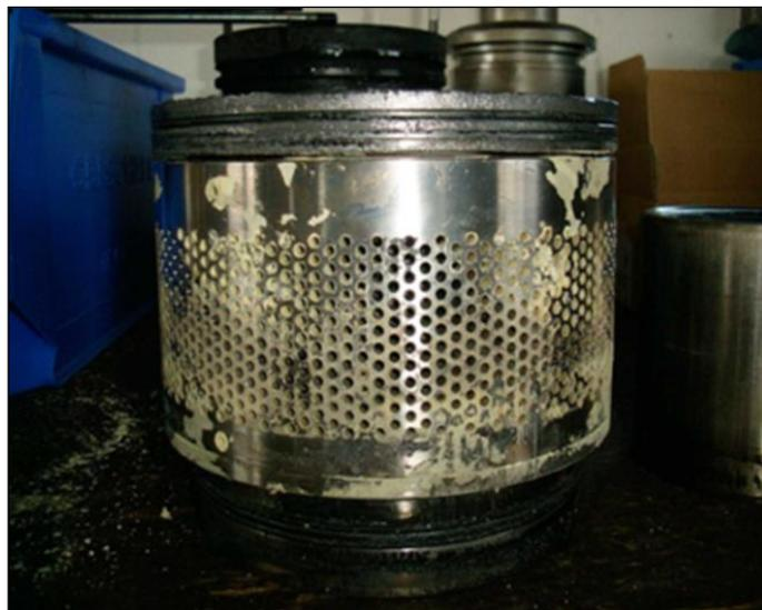
*Figure 1: Sulphur deposits in control valve of UGS*
