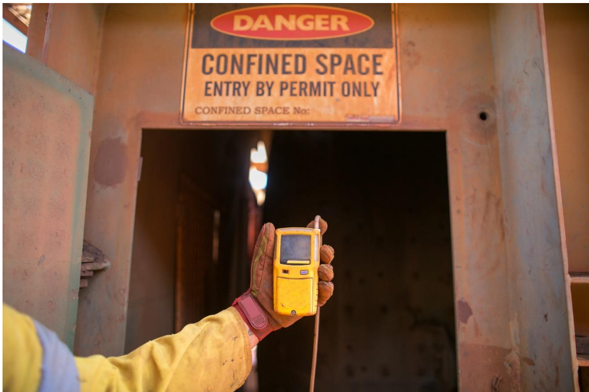
Figure 2: Control of the atmosphere before entering in a confined space
