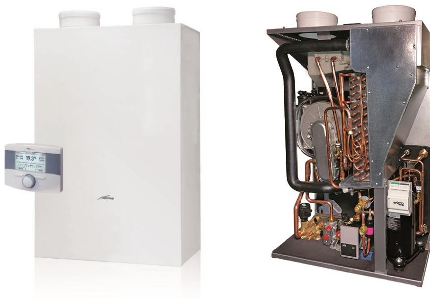
Figure 3 – The Murelle Revolution 30 Hybrid Heating System combines a 24 kW gas condensing boiler and a 4 kW thermal air/water heat pump in a single product and does not require an outside unit. The unit measures only 900 x 600 x 390 mm. Image copyright: Sime [8].
