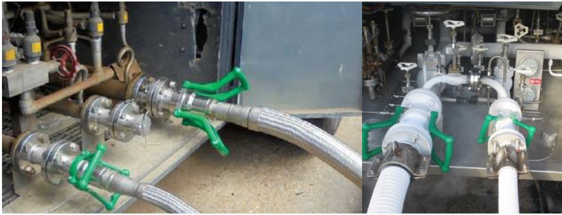
Figure 2 - Tank unit – LNG terminal connections
