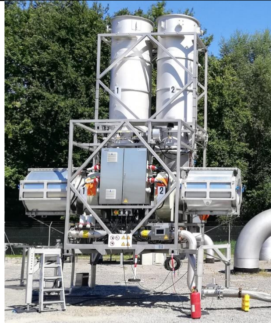
Figure 6 – Lambda mobile flare system
