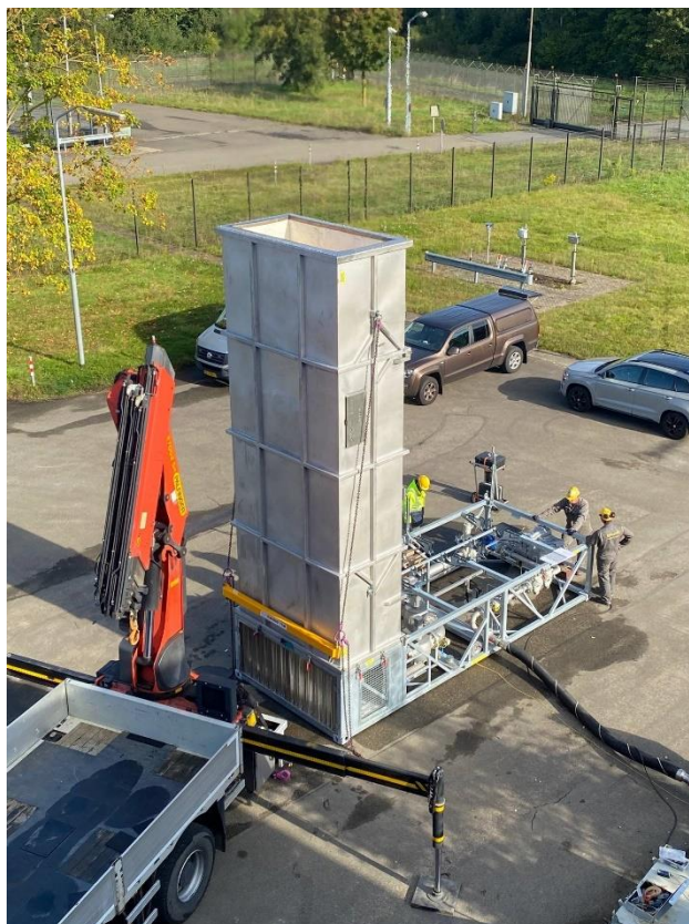
Figure 3 – Enwell BV enclosed mobile flare 1200 m 3 N/h (Gasunie)
