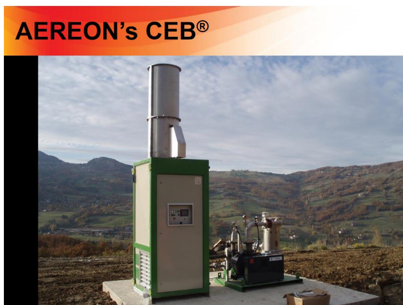
Figure 5 – Aereon flare unit for permanent unattended operation
