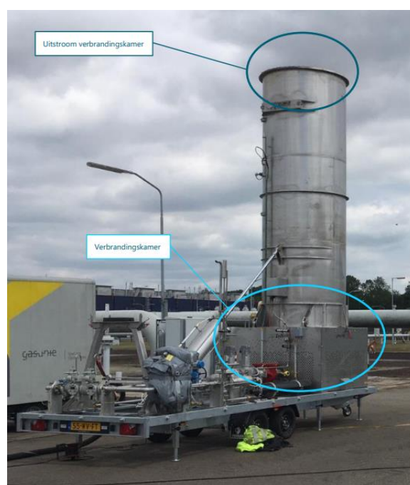
Figure 2 – Enwell BV enclosed mobile flare 500 m 3 N/h (Gasunie)
