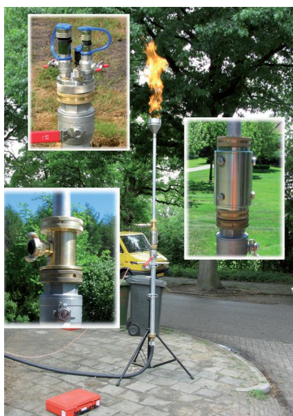
Figure 1 – Esders open flame flaring system
