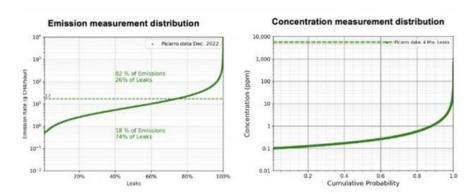
It is important to ensure that large leaks (above 1000 ppm for type 2 LDAR) are detected.
